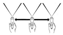
Begin spraying by pulling the Trigger and move the Spray Gun in the direction you want to spray. Start your pass from off the edge of the piece; then continue off the edge of the piece on the other end before releasing the Trigger. Between each successive pass, overlap by 50%.
