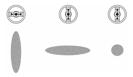
A) Loosen the Collar #1. Turn the Aircap #2 to the horizontal position. This setting produces a vertical spray pattern. Always make sure the Collar is snug tight.
