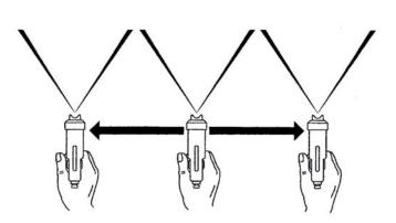
Start moving the spraygun in the direction you want to spray and press the trigger. Between each successive pass, overlap by about a quarter.
