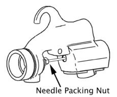
It is a good idea to apply Light Machine Oil or Vaseline to the Needle Shaft where it passes through the Needle Packing Nut and work it in and out by pulling the Trigger back and forth. This will lubricate the Needle Packing #12.
